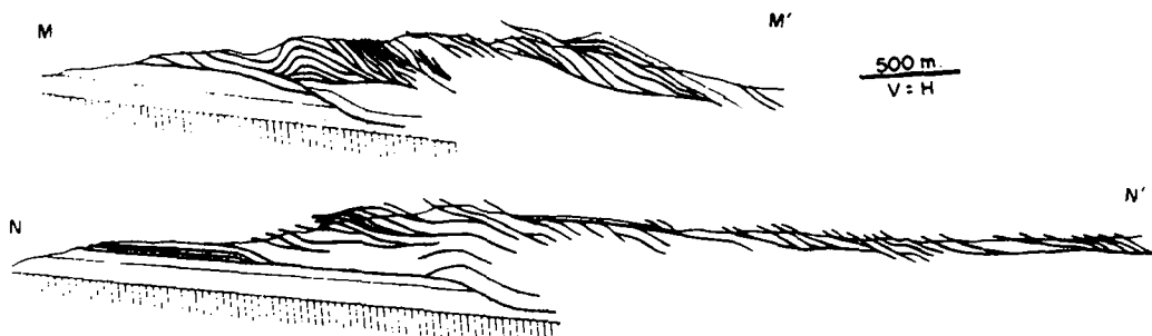
Fig. 7. Cross sections M-M' and N-N' drawn through the Conamheall duplex. Pipe Rock is unornamented, the fine stipple is An t-Sron Formation. All thick lines are thrusts, movement to NNW.
